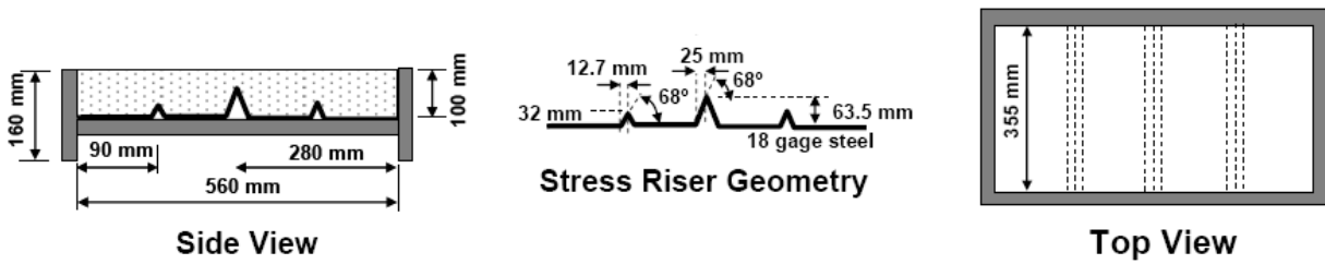
Figure 3 – Geometry of the specimens used for concrete plastic shrinkage investigation (25.4 mm = 1 in) [6].
